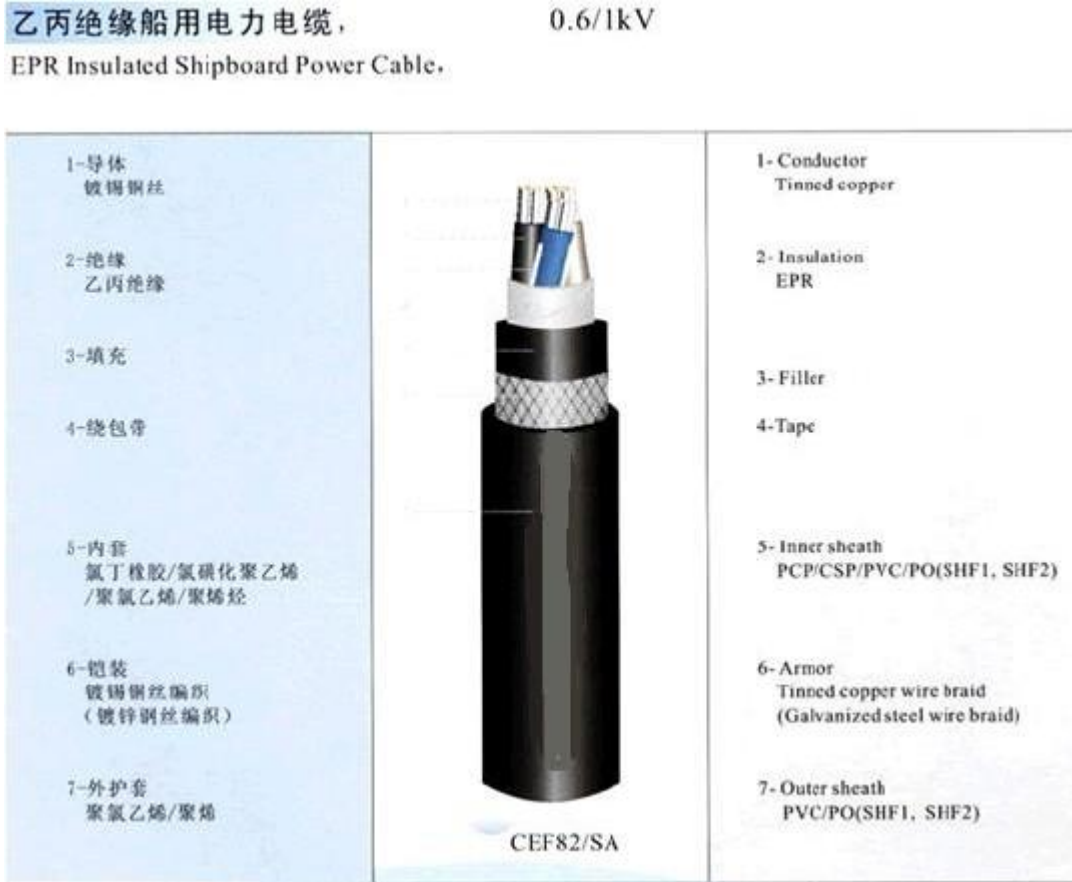
Figure 5.5.3.3(1) B-C insulated marine power cable
