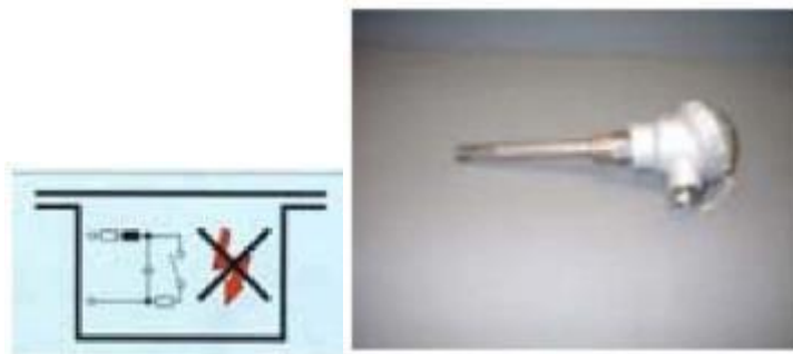
Figure 5.5.3.1(3)① Intrinsically safe and PT-100 temperature sensor
